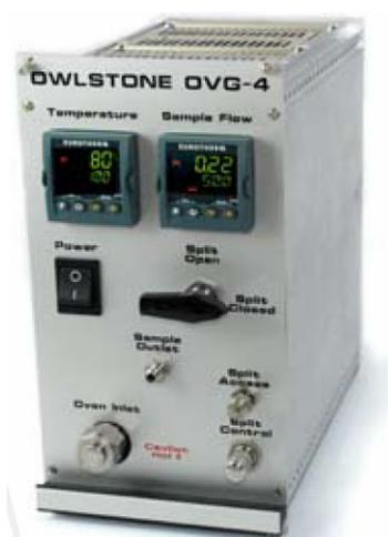
**Figure 3.11** Owlstone vapour generator (OVG) 4.
