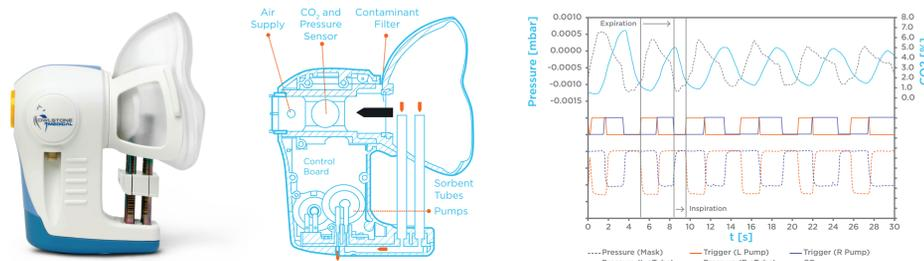
Figure 1. The ReCIVA Breath Sampler (left and middle panel) enables reliable, reproducible collection of breath VOCs and pre-concentration for enhanced sensitivity. Pressure and CO<sub>2</sub> sensors in ReCIVA provide real-time monitoring of the patient's breathing, allowing different breath fractions to be sampled in a single collection event if desired (right panel).
