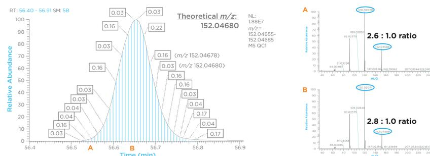
Figure 3. Sub-1 ppm mass accuracy is achieved across a 44 scan-wide chromatographic peak (100 ppm sample; left panel). Identical relative fragment ion ratios are observed even at high concentrations (200 ppm sample; right panel).
