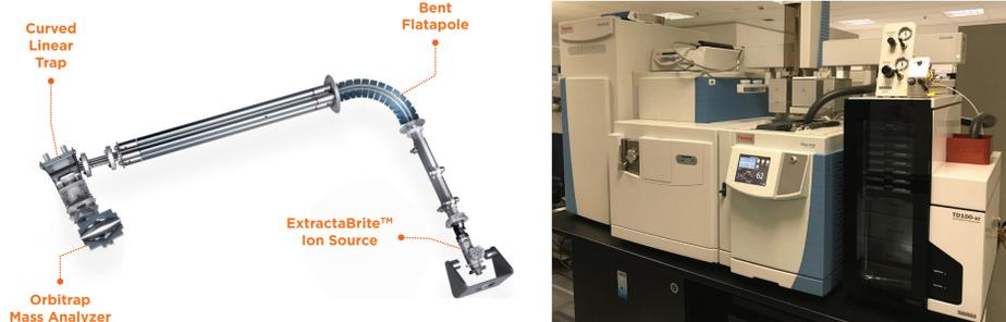
Figure 2. Internal lay-out of the Exactive GC Orbitrap analyser (left panel) and TD-GC-Orbitrap setup used in this study (right panel)
