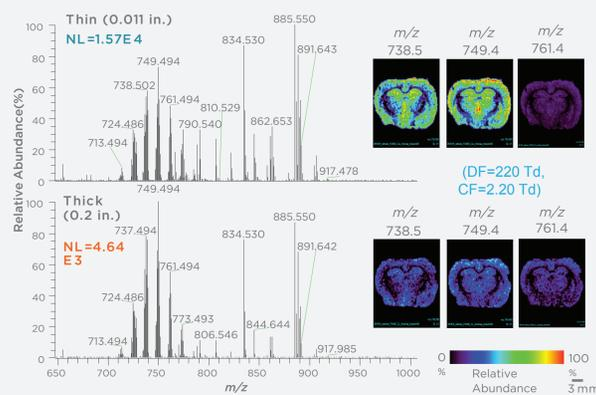
Figure 6. Comparison of thickest and thinnest walled capillaries with FAIMS voltages set to transmit cardiolipins
