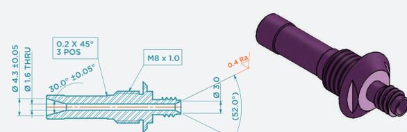
Figure 9. Customised 1/16" Swagelok nut DESI-FAIMS inlet design
