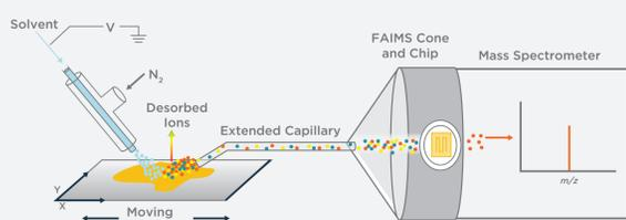
Figure 2. Schematic representation of selective FAIMS transmission of ion of interest using DESI-FAIMS-MS
