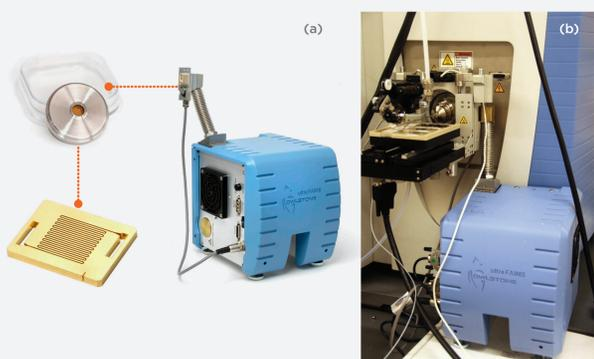
Figure 3. (a) ultraFAIMS T1 device and (b) installed on Q-Exactive with 2D Omni Spray
