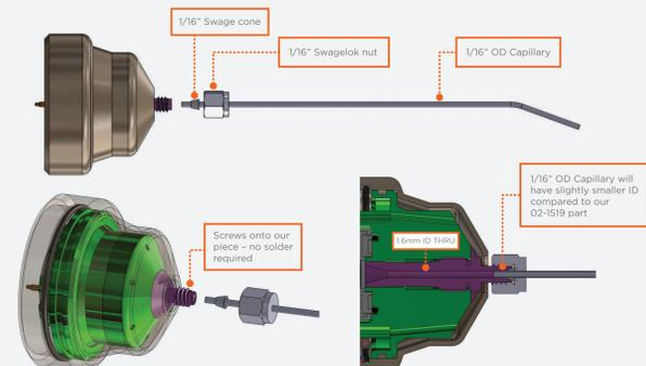
Figure 8. 1/16" Swagelok nut DESI-FAIMS interface design (DI2)
