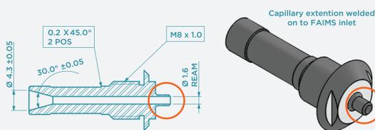
Figure 4. Standard FAIMS inlet design indicating part needing extension
