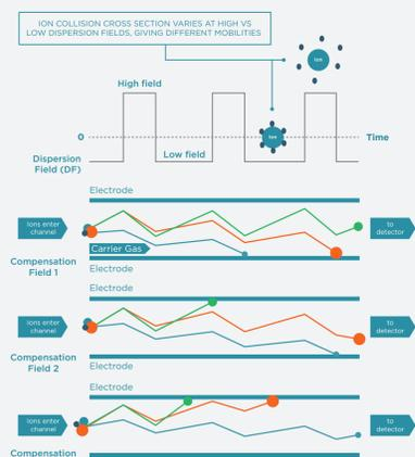
Figure 1. FAIMS separates ions according to field-induced changes in their collision cross section
