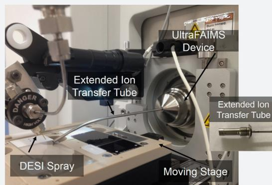
Figure 5. (a) ultraFAIMS T1 device and (b) installed on Q-Exactive with 2D Omni Spray
