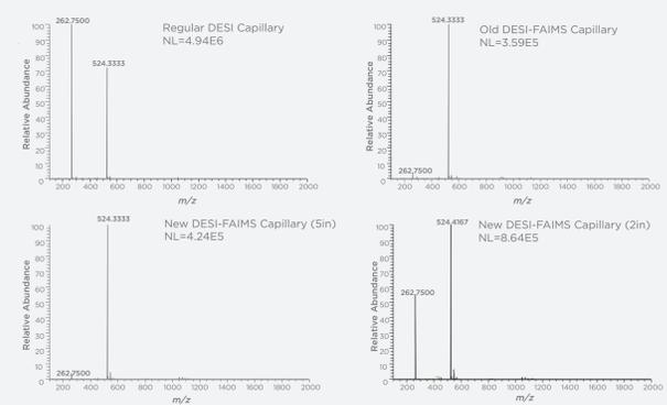
Figure 11. MRFA signal intensity between DESI, DI1 and 5" and 2" capillary DI2 inlets
