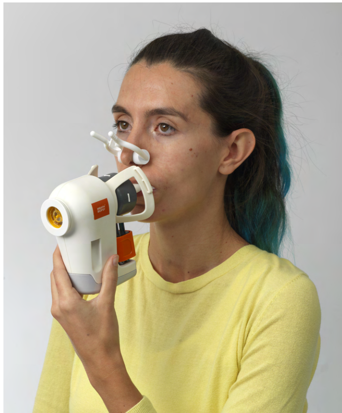
Figure 3: A demonstration of the ReCIVA Breath Sampler device in use with the coupled nose clip. In certain circumstances a mask can be used instead.
