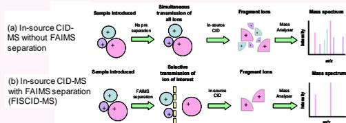
Figure 1. Schematic representation of in-source CID-MS and FISCID-MS data acquisition.
