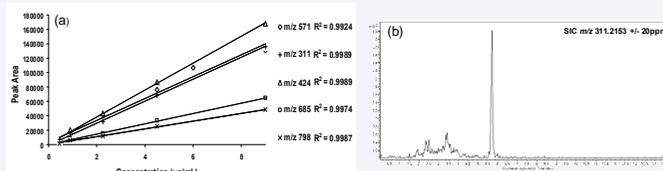
Figure 4. (a) Calibration graphs for the LC-FISCID-MS analysis of the FAIMS-selected (CV 1.75-1.85 V)  $[\text{M}+2\text{H}]^{2+}$  precursor ion ( $m/z$  571) and four product ions ( $m/z$  311, 424, 685 and 798) of gramicidin S spiked in human plasma tryptic digest and (b) LC-FISCID-MS chromatogram for  $m/z$  311 fragment ion.
