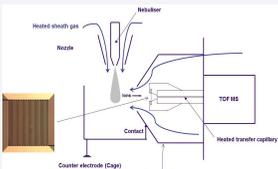
Figure 2. Schematic diagram of the miniaturised FAIMS chip interfaced with a TOF mass spectrometer.
