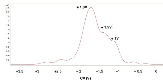
**Figure 3** EIC for  $m/z$  687 ( $[M+18H]^{18+}$  charge state) of cytochrome C, indicating the presence of at least 3 isobaric species of differing differential mobility.
