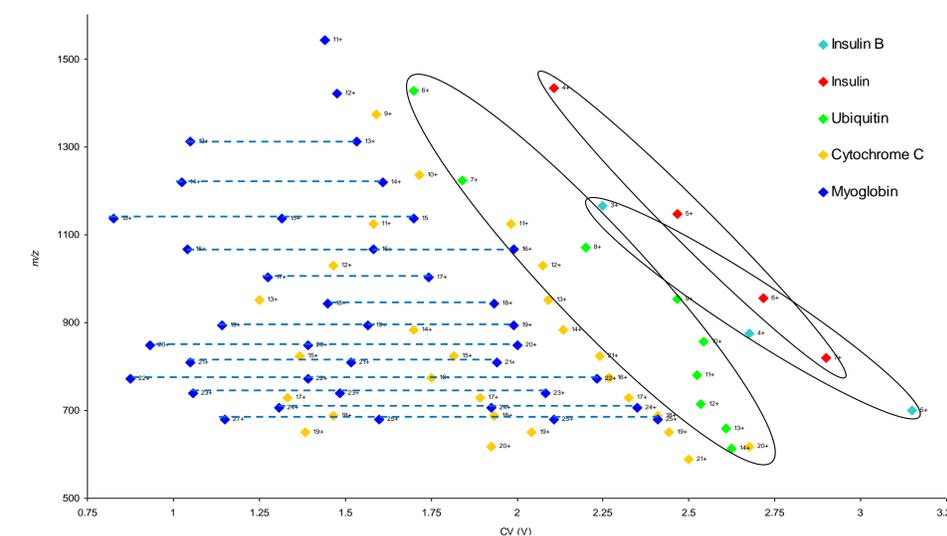
**Figure 4** Plot of  $m/z$  vs. CV for all studied proteins. Multiple components of the same  $m/z$  of myoglobin are observed demonstrating the broad CV distribution of suspected conformations.
