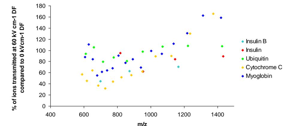
**Figure 5** A plot of  $m/z$  vs. protein transmission. Enhanced transmission is observed for higher molecular weight proteins of lower charge state.
