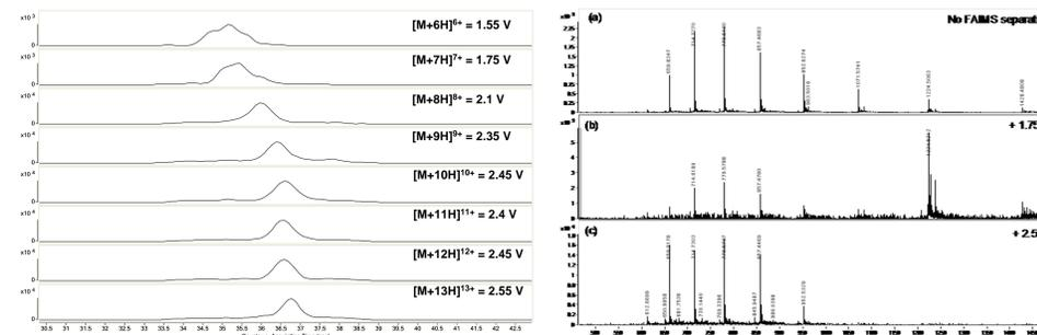
**Figure 2** Extracted ion chromatograms (EIC) showing FAIMS-MS separation of multiple charge states of bovine ubiquitin and ubiquitin mass spectra (a) No FAIMS (b) +1.75 V CV showing preferential transmission of the +7 charge state ( $m/z$  1224) and (c) +2.55 V CV showing simultaneous transmission of +9 to +13 charge states at the expense of lower charge state species.
