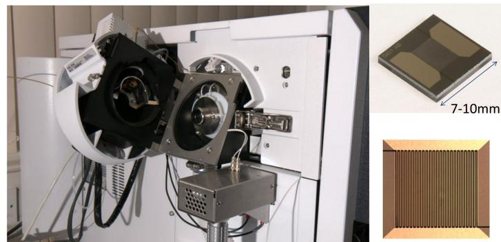
**Figure 1** Prototype chip-based FAIMS device installed on Agilent TOF, with close-ups of the FAIMS chip
