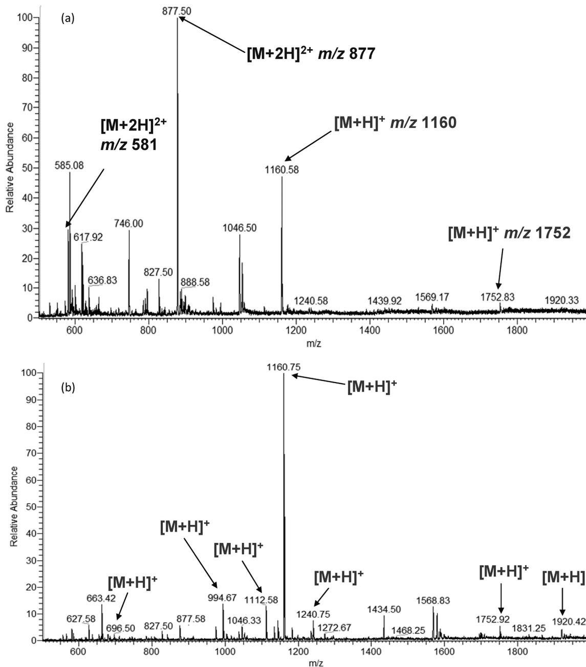
**Figure 7.** (a) Mass spectrum of the AAG tryptic digest with no FAIMS separation. (b) The mass spectra obtained with the CV window set to +1.5-+1.7 to isolate the singly charged ions.
