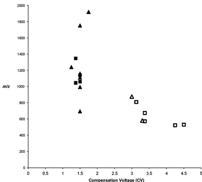
**Figure 5.** Compensation voltage vs  $m/z$  plot of singly and doubly charged standard and tryptic peptide ions: ■, singly charged standard peptide ions; ▲, singly charged tryptic peptide ions; □, doubly charged standard peptide ions; △, doubly charged tryptic peptide ions.
