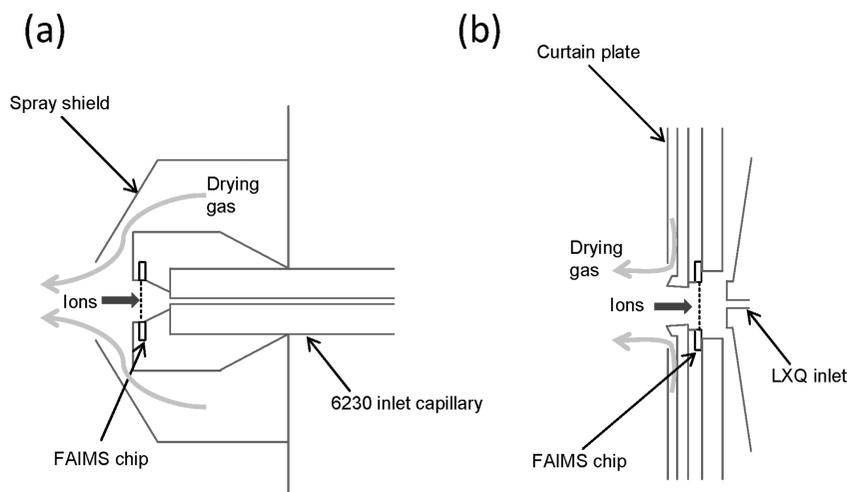
**Figure 1.** Schematic diagrams of (a) the ultra-FAIMS chip mounted into the chip cartridge and housed within the Thermo “Ion Max” ion source and (b) located within the spray shield of the Agilent Jet Stream source.
