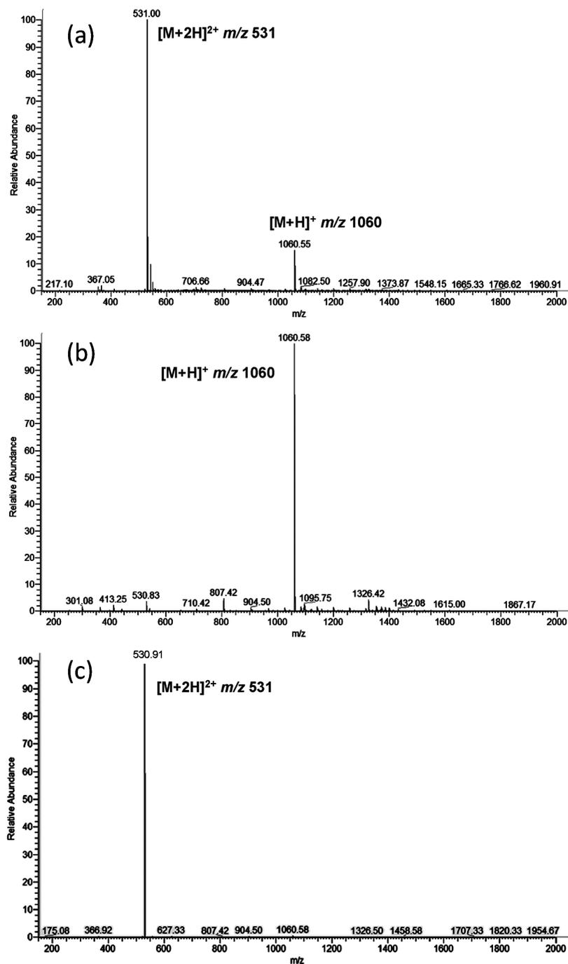
**Figure 2.** FAIMS-MS charge state separation of bradykinin ions. (a) Ion trap mass spectrum without FAIMS separation (S/N ratio 100:1 ( $m/z$  1060); 1000:1 ( $m/z$  531)). (b) Selective enhancement of the  $[M+H]^+$  ( $m/z$  1060) ion at a CV of +1.4 V (S/N ratio 1000:1) and (c) selective enhancement of the  $[M+2H]^{2+}$  ( $m/z$  531) ion at a CV value of +3.5 V (S/N ratio 10 000:1).
