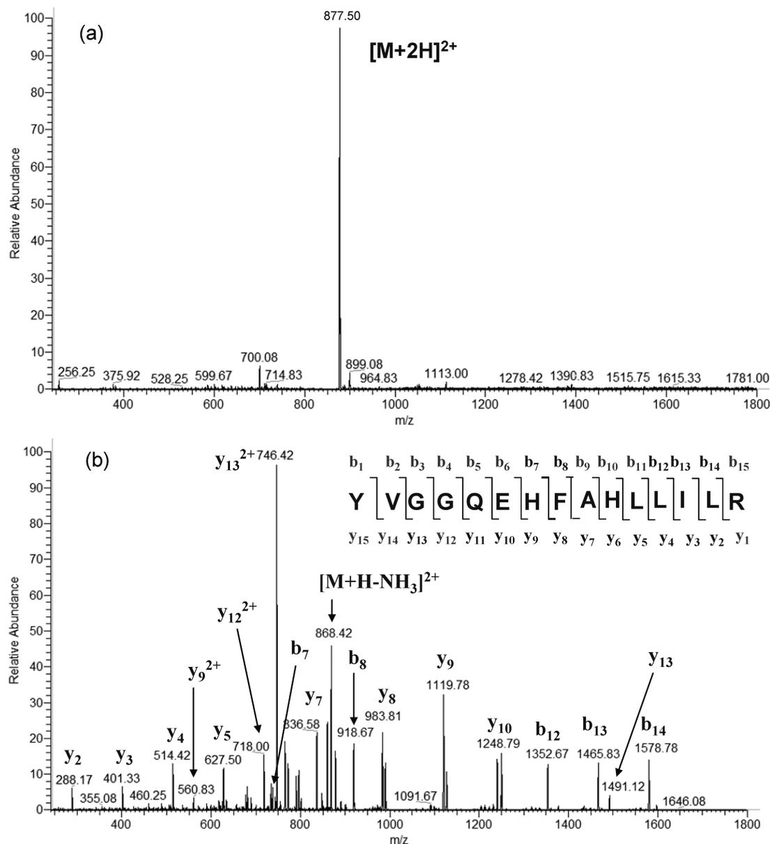
**Figure 8.** (a) Selective enhancement of the  $m/z$  877 ion from the AAG tryptic digest and (b) the ion trap MS/MS spectrum of the  $m/z$  877 ion.
