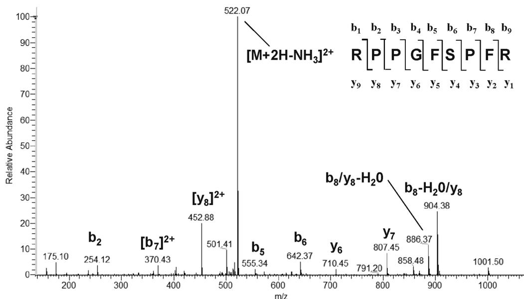
**Figure 6.** Ion trap tandem mass spectrometry of the ultra-FAIMS selected  $[M + 2H]^{2+}$  ion of bradykinin ( $m/z$  531).
