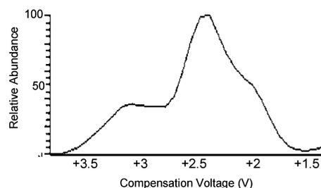
**Figure 3.** CV scan for the FAIMS-MS ion trap analysis of the bradykinin  $[M + 2H]^{2+}$  ion at a DF of  $60 \text{ kV cm}^{-1}$ .
