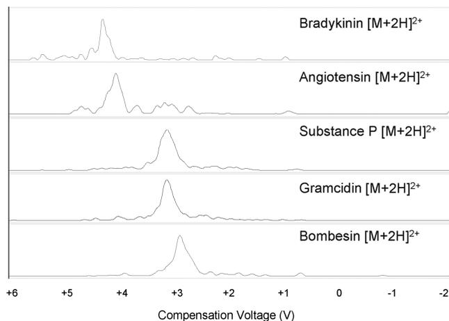
**Figure 4.** FAIMS-TOF-MS analysis of a mixture containing bradykinin ( $m/z$  530.7), angiotensin ( $m/z$  523.7), substance P ( $m/z$  674.3), gramicidin S ( $m/z$  571.3), and bombesin ( $m/z$  810.4) at a DF of  $60 \text{ kV cm}^{-1}$ .
