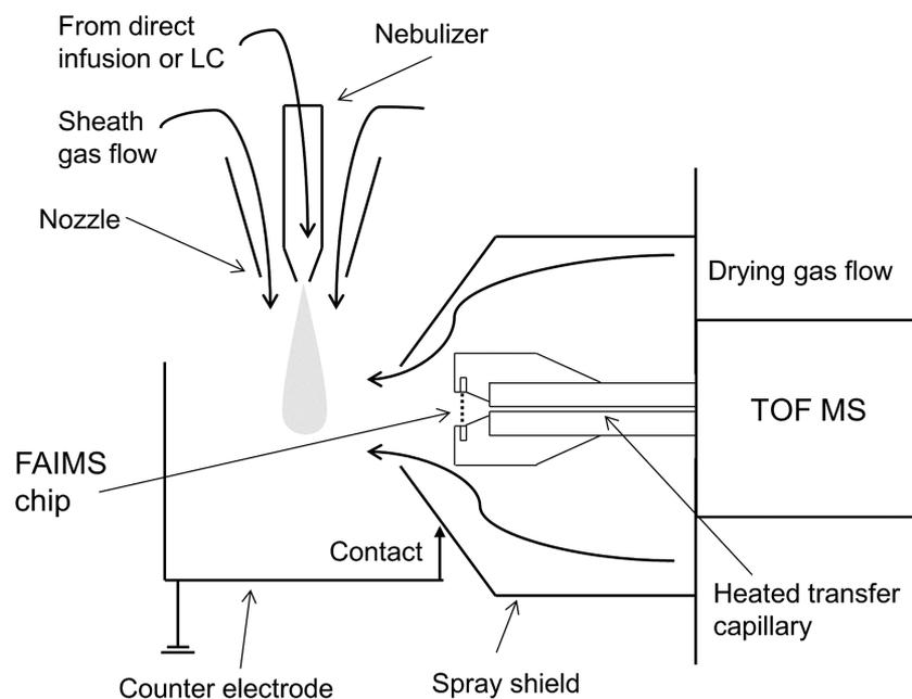
**Figure 1.** Schematic diagram of the FAIMS-MS interface.
