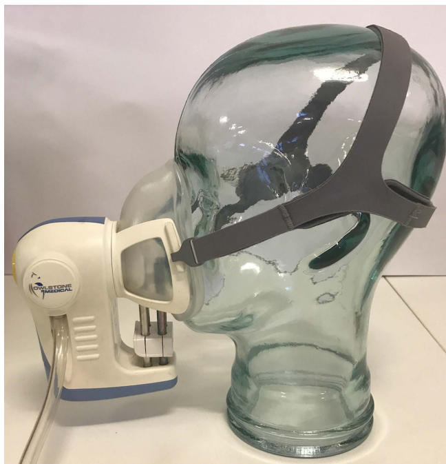
Figure 1. Collection system used to assess environmental contamination Glasshead (AMP3 Ltd, Aldershot, UK) and ReCIVA device (Owlstone Medical, Cambridge, UK).
