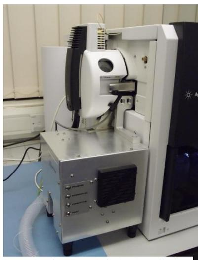
Figure 2: UltraFAIMS device installed on Agilent 6230 TOF
