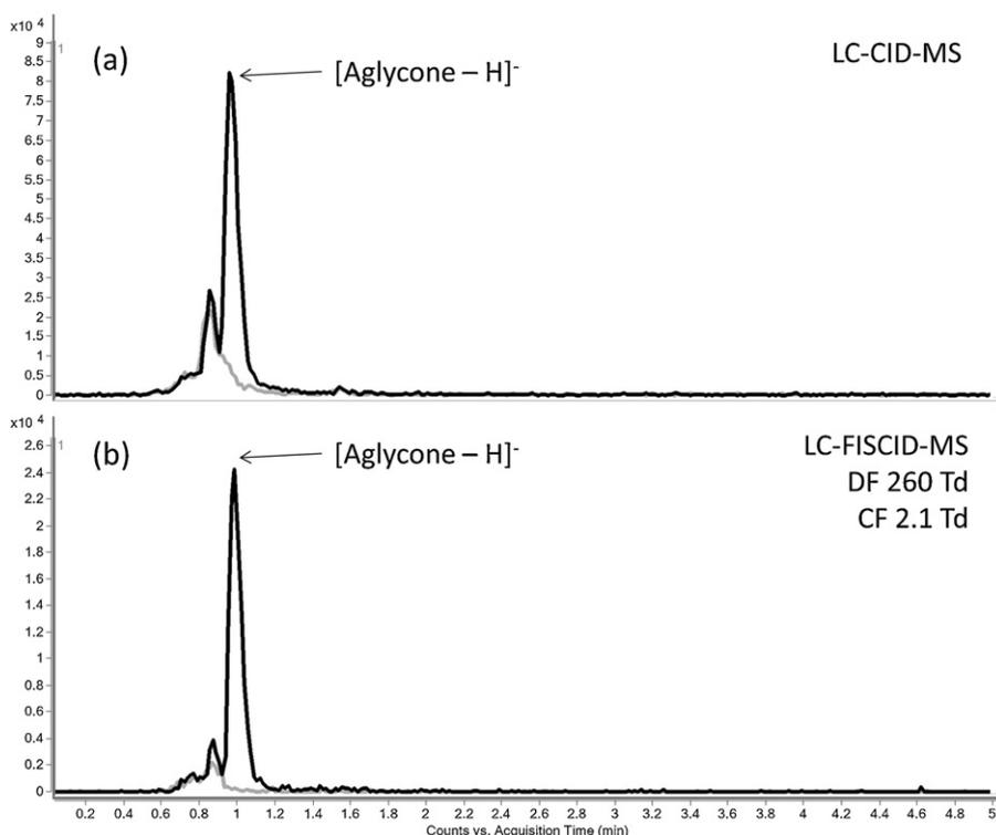
**Fig. 5.** Selected ion chromatograms ( $m/z 205 \pm 0.02$ ) of the  $[\text{Aglycone-H}]^-$  for the urine blank (grey) and IAG (black) spiked into urine ( $3.9 \mu\text{g/ml}$ ) by (a) UHPLC-CID-MS and (b) UHPLC-FISCID-MS.
