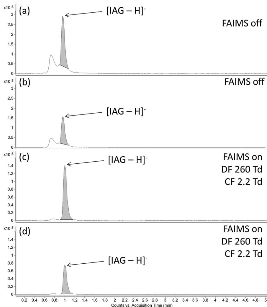
**Fig. 3.** Selected ion chromatograms ( $m/z$  381) for IAG (highlighted) spiked into urine ( $0.55 \mu\text{g/ml}$ ) analysed by UHPLC–MS (FAIMS off) using a mass window of (a)  $m/z$   $381 \pm 0.02$  and (b)  $m/z$   $381 \pm 0.008$ ; and by UHPLC–FAIMS–MS (FAIMS on) with selective transmission of IAG (DF 260 Td, CF 2.2 Td) using a mass window of (c)  $m/z$   $381 \pm 0.02$  and (d)  $m/z$   $381 \pm 0.008$ .
