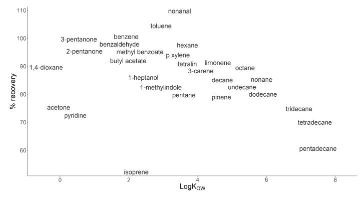
Compared the recovery of each VOC in the standards mix in the dry and wet gas samples
