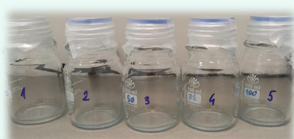
Acetone calibration gas standards
