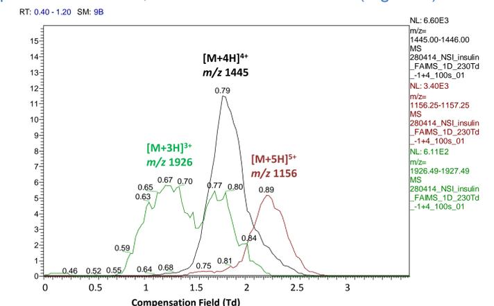
Figure 6. FAIMS spectra of insulin  $[M+3H]^{3+}$ ,  $[M+4H]^{4+}$  and  $[M+5H]^{5+}$  at 230 Td
