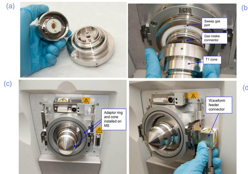
Figure 3. Second design iteration of microscale FAIMS chip. (a) Chip in the revised chip cone. (b) Chip interface fits over the spray cone of Thermo Scientific LTQ Orbitrap or Exactive series mass spectrometer. (c) FAIMS interface in place, with adaptor ring allowing attachment of any standard ionisation source. (d) Waveform feeder connector fits into adaptor ring to bring FAIMS waveform from controller module to chip.
