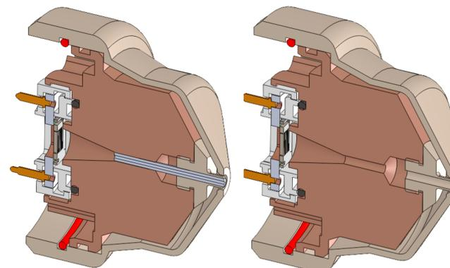
Figure 4. CAD drawings of (a) 0.8mm and (b) 1.6mm bore diameter chip cone
