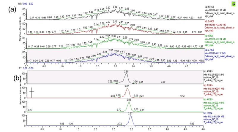
Figure 5. FAIMS spectra of ultramark 1621 oligomers at 295 Townsend (Td) dispersion field (DF) with (a) the narrow and (b) the wider bore diameter chip cone.
