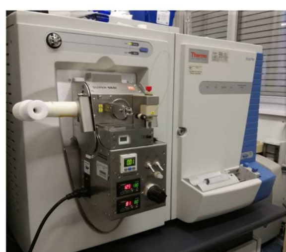
SUPERSESI (FOSSILIONTECH) COUPLED TO THERMO LTQ ORBITRAP ELITE
