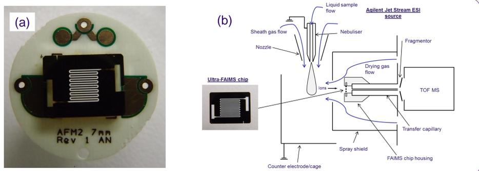
Figure 2. (a) Photograph of the miniaturised chip-based FAIMS device and (b) Schematic diagram of FAIMS interfaced with the TOF-MS.
