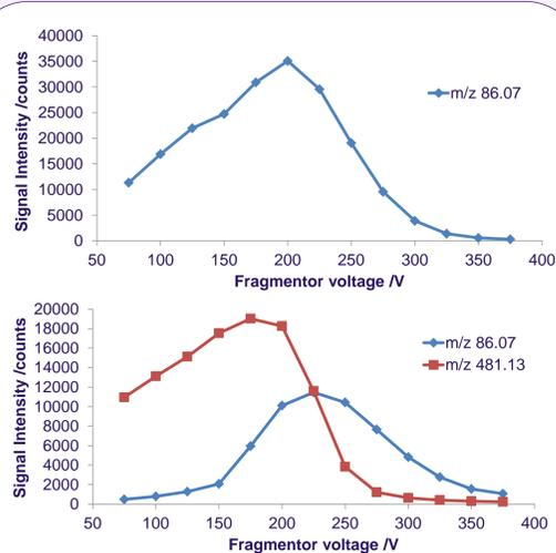
Figure 3. a plot of intensity of  $m/z$  86.07 (blue) and 481.13 (red) in (a) NMP standard; and (b) Cefepime sample without NMP added
