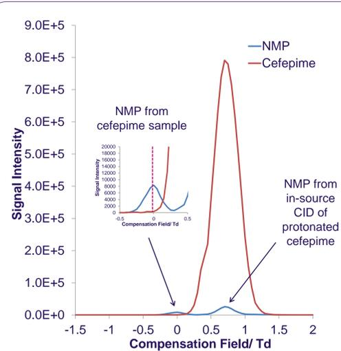
Figure 4. FAIMS CF spectrum of NMP ( $m/z$  86.07, blue trace) and cefepime ( $m/z$  481.13, red trace) for a Cefepime sample spiked with NMP (0.1% w/w) at a DF of 180 Td. Insert, the spectrum in the CF range -0.5 to +0.5 Td.
