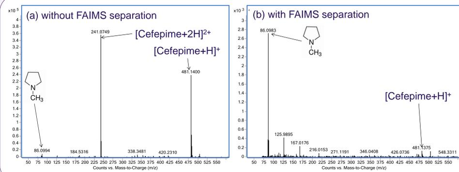
Figure 5. Mass spectra of NMP (0.05  $\mu\text{g}/\text{ml}$ ) in cefepime (50  $\mu\text{g}/\text{ml}$ ): (a) without FAIMS separation and (b) with the FAIMS set to CF 0 Td, DF 180 Td to transmit NMP.
