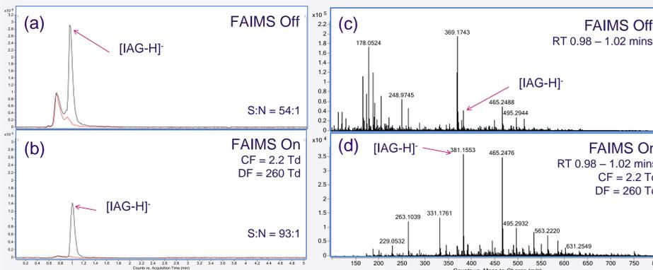
Figure 3. Overlaid EICs (m/z 381 ± 0.02) for urine blank (red trace) and IAG (black trace) spiked into urine (0.55 µg/ml) with (a) FAIMS off, and (b) FAIMS on. Mass spectra of [IAG-H]<sup>-</sup> LC peak with (c) FAIMS off, and (d) FAIMS pre-selection of [IAG-H]<sup>-</sup>
