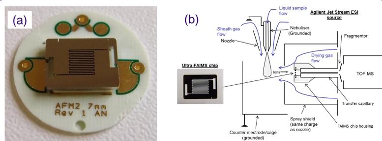
Figure 1. (a) The miniaturised chip-based FAIMS and (b) interfaced with the TOF-MS.
