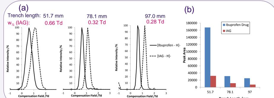
Figure 2. (a) FAIMS-MS CF scans of ibuprofen and the IAG metabolite with different trench lengths and (b) a plot of CF peak area against trench lengths (n = 6)
