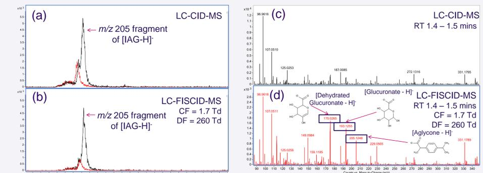
Figure 4. Overlaid EICs (m/z 205) for urine blank (red trace) and IAG spiked urine (3.9 µg/ml) (black trace) using (a) LC-CID-MS and (b) LC-FISCID-MS (FAIMS-selected [IAG-H]<sup>-</sup> ion). Mass spectra of [IAG-H]<sup>-</sup> LC peak with (c) FAIMS off, and (d) FAIMS selecting [IAG-H]<sup>-</sup>
